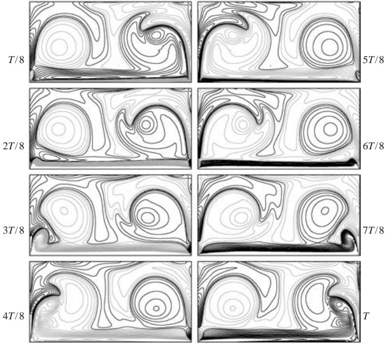
FIGURE 11. Contours of z -vorticity of the basic state at ( St = 100 , Re = 1212 ) (which is unstable to mode QP) over one forcing period, T .
